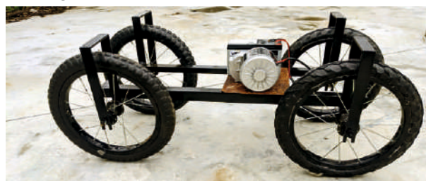
Fig. 3.5.10: Fabricated frame of multipurpose vehicle
